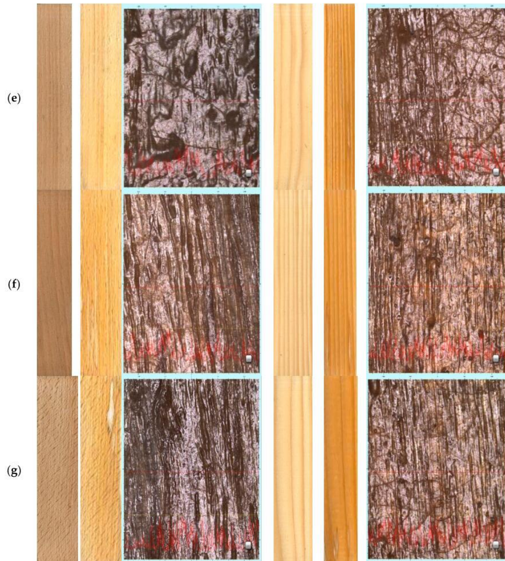
Figure 1. Beech (left) and spruce (right) wood samples before (0.w.) and after accelerated weathering (AW) (6.w.). (a) Reference native wood (R-R); (b) acrylic coating on untreated wood (R-A); (c) acrylic coating on caffeine treated wood (5-A); (d) acrylic coating on wood treated with 10% FN-NANO ® (1-A); (e) acrylic coating on wood treated with 15% FN-NANO ® (2-A); (f) acrylic coating on wood treated with a mixture of 10% FN-NANO ® and 1% of caffeine (3-A); (g) acrylic coating on wood treated with a mixture of 15% FN-NANO ® and 1% of caffeine (4-A). Note: The real observed area of microscopic picture was 2500 \mu\text{m} \times 2500 \mu\text{m} using 108-fold magnification.
