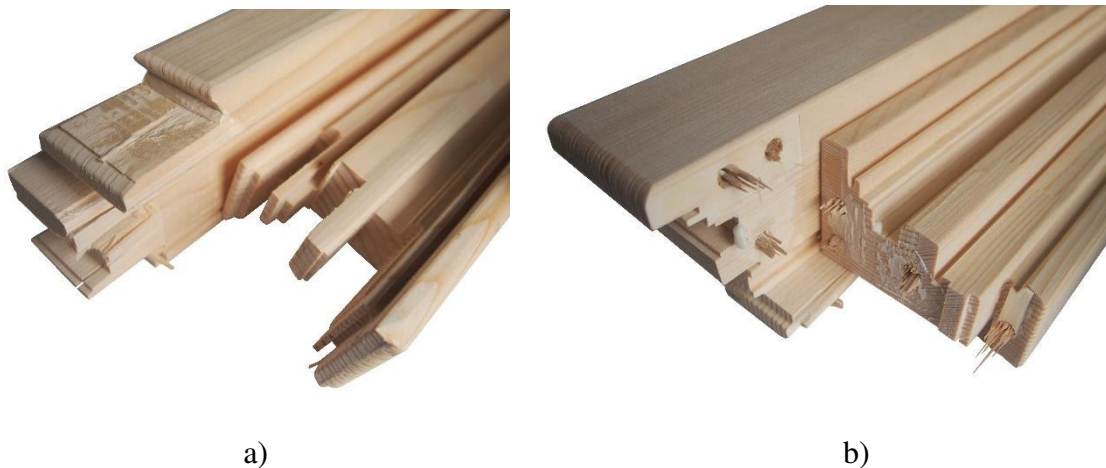
Fig. 5. Example of failure modes in compression: triple tenon and mortise (a) and dowel joint (b)
