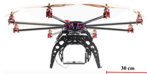
Figure 6. Scaled image that illustrates the actual size of the octocopter Steadi Drone EI8HT RTF that was used for the acquisition of aerial images.
