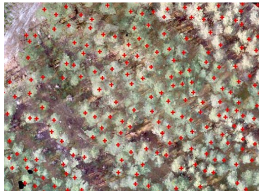
Figure 3. The applied method of local maxima seeds for the derivation of tree heights (red crosses show the detected treetops by the local maxima approach).
