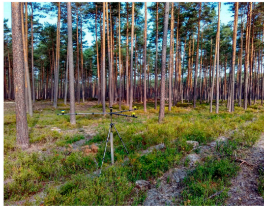
Figure 3. Illustration of Postex technology for georeferencing the position of each plot.
