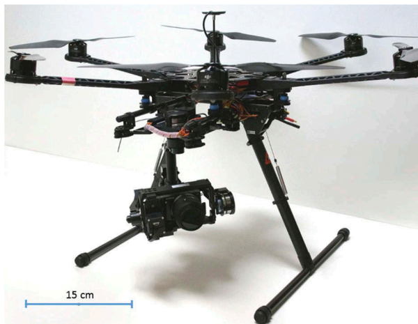
Figure 3. This is a scaled image that illustrates the actual size of the multirotor UAV (DJI S800) that was used for photograph acquisition (source: Přemysl Janata).
